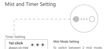
please press switch for 2 seconds 1 hour mist until indicator blinks: Intermittent mist (30 sec. on /30 sec. off) ← Continuous mist
